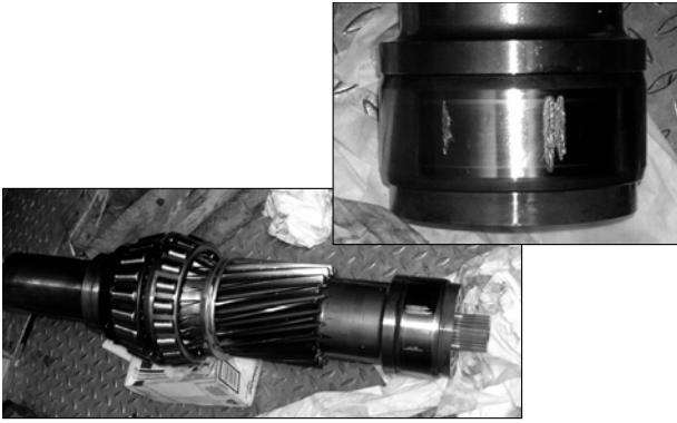
Fig.5: On the inner race the expected defects are visible. The repair was carried out in early May. Three month in advance the problem was detected in an early state. The conclusions allowed shifting of the repair into a low wind period.
